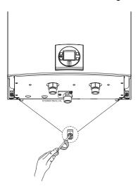
Fig. 3 Loosen the two screws
